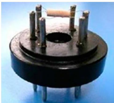
Figure 3. Photograph of the gas sensor.
